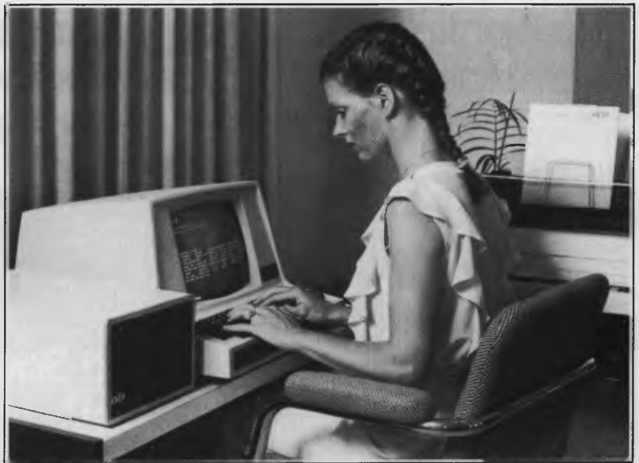
A typical personal computer set-up: dual floppy disk drive, terminal and keyboard, printer (in this case letter quality).
