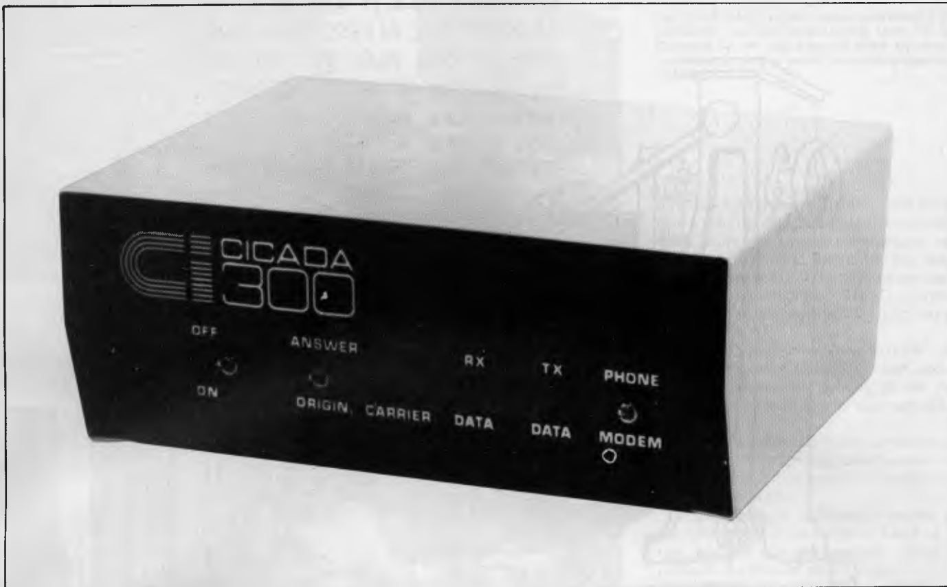
A basic 300 baud modem. This device connects the computer to the telephone line directly.
